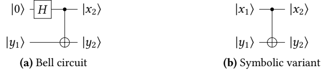
Figure 2. A conventional quantum circuit for generating a Bell state (a); its classical symbolic variant (b)
